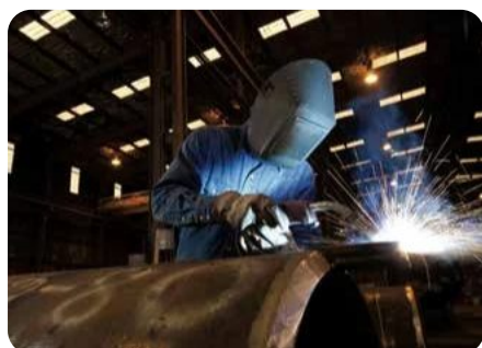
Welder in a helmet welding a large steel vessel shell in the World Heat Cylinders factory
