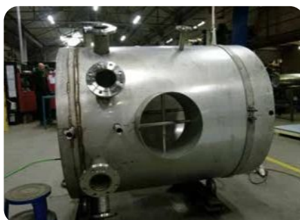
A large stainless steel calorifier shell with flanged connections and an inspection
