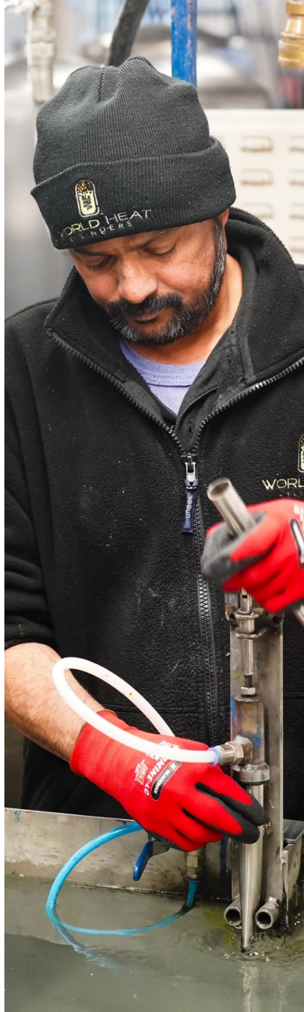
Leak testing a fabricated assembly in the World Heat Cylinders workshop
