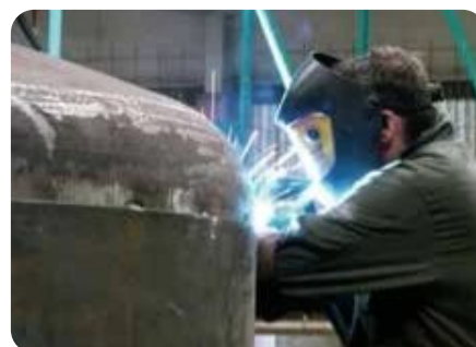
Welder at work on a large steel vessel at the World Heat Cylinders factory
