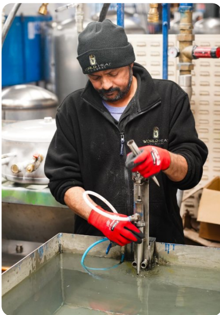
Leak testing a fabricated assembly in the World Heat Cylinders workshop
