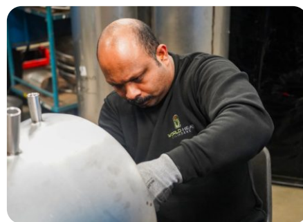
Technician fitting a stainless steel domed end at the World Heat Cylinders factory
