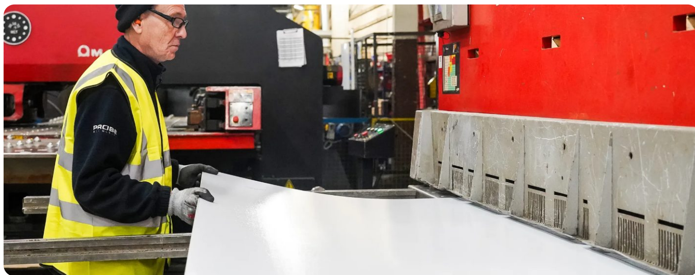
Operator feeding a steel sheet into the press brake
