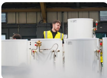
Finished domestic hot water cylinders on the production floor
